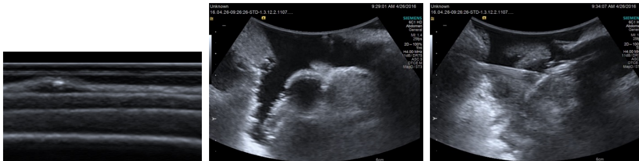
Figure 13: Left: The skin, subcutaneous fat, and urethane joint capsule tissue mimics. Center: The acetabulum and femoral head. Right: A needle piecing the joint capsule space.
