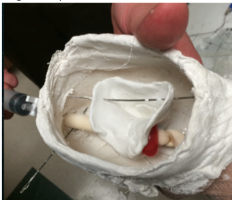
Figure 1: Dr. Halanski's initial prototype. The model is made from a plaster mold. The inside of the model is hollow so it can accommodate a balloon containing fluid [8].
