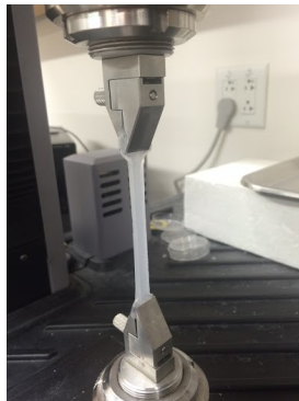
Figure 11: A skin mimic sample undergoing tensile testing.
