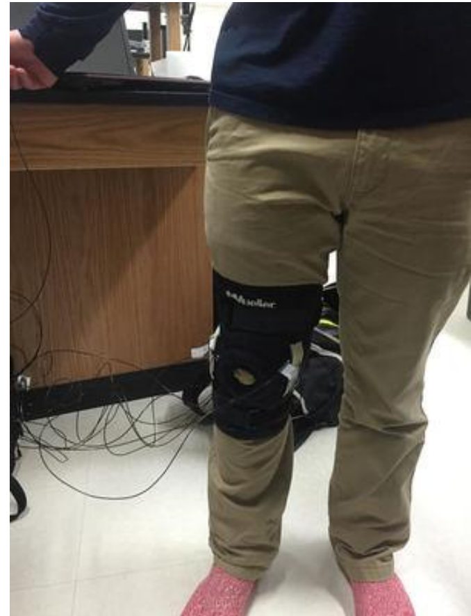
Figure 17: FSRs are attached to the hinges inside the knee brace being worn by a team member.
