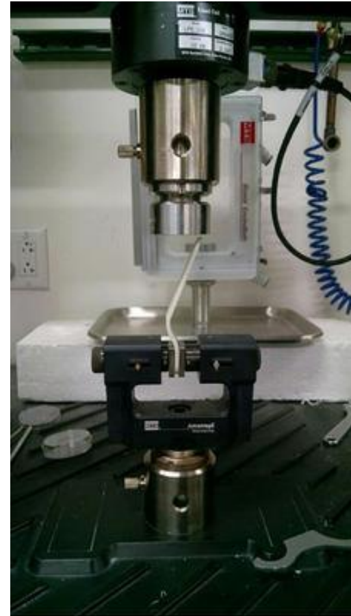
Figure 16: Static testing setup of the Y-arm design in the MTS machine.
