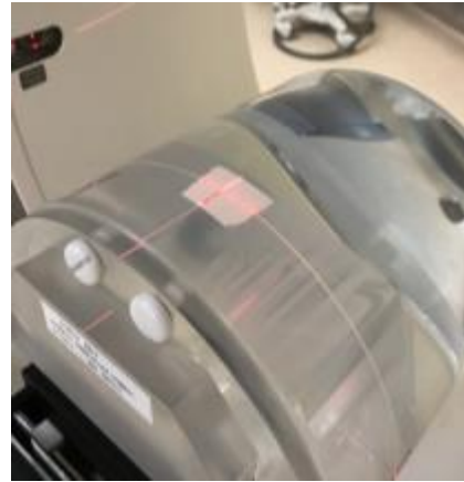
Figure 18. Laser Levelness and Orthogonality Test. A phantom is used to assess the lasers by checking if they align with markers at 3, 9, and 12 o'clock positions.
