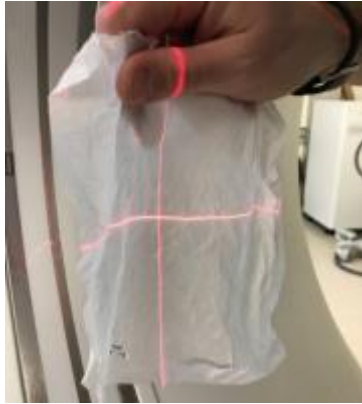
Figure 17. Tissue Test. A test performed to check the coincidence of the lasers. If the lasers are not coincident, the difference in millimeters is recorded.
