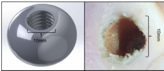
Figure 8: On the left is a Solidworks model of the threaded recipient site. On the right is a threaded recipient site on a condyle bovine femur
