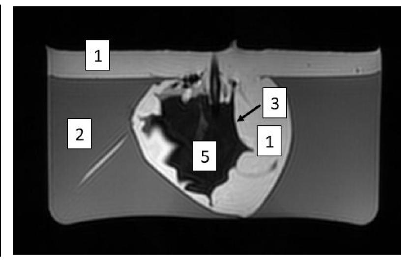
Figure 2: MR image of prototype before clot aspiration (left) and after aspiration (right). Hydrogel(1) filling in the void as plasma aspiration is visible. Materials of the images are as following:
