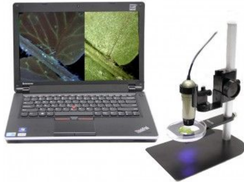
Figure 4. Dino-Lite Fluorescent Microscope [8]. A small hand held microscope that connects to your computer.
