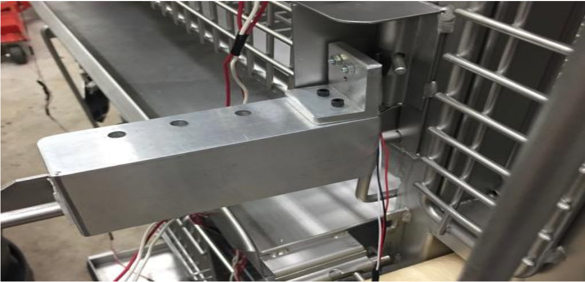
Figure 11: Final clamp design attached to monkey cage
