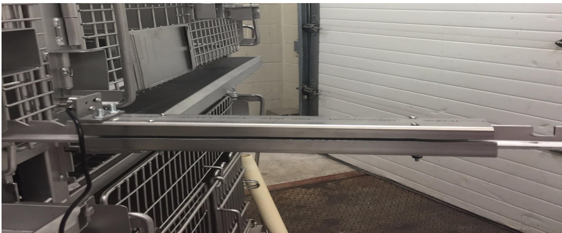
Figure 3: Original clamp design depicted attached to the monkey cage
