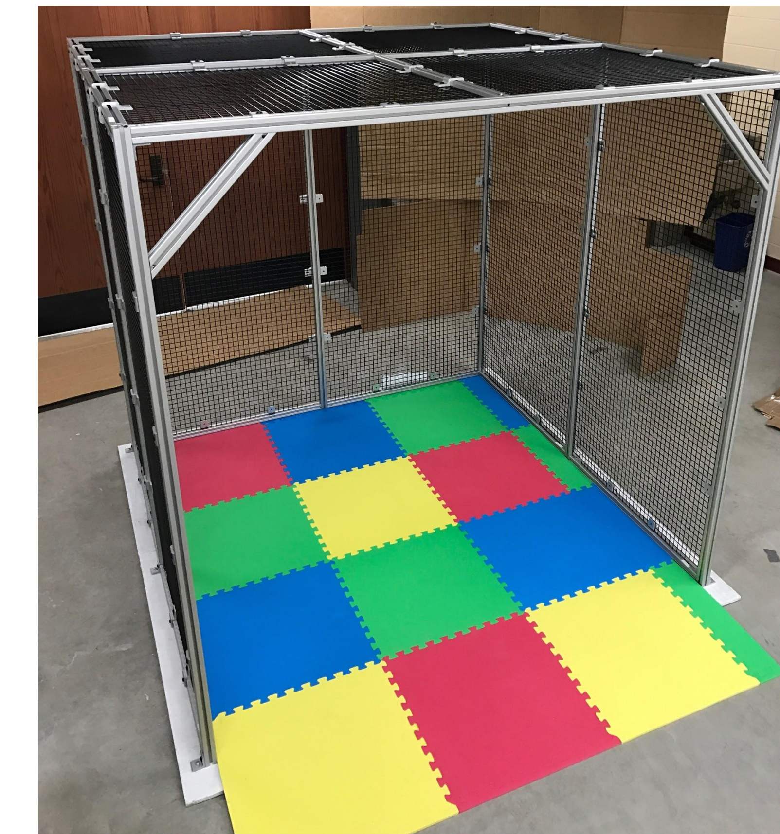
Figure 2: The final design for UCP's spider cage which has a frame made of 80/20, wire mesh for resistance band attachments, and padded flooring.
