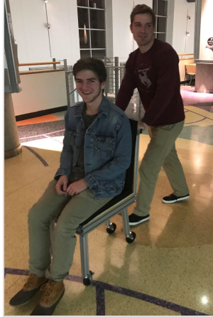
Figure 14 (left): Static load test with 305 lbs loaded onto the chair.
