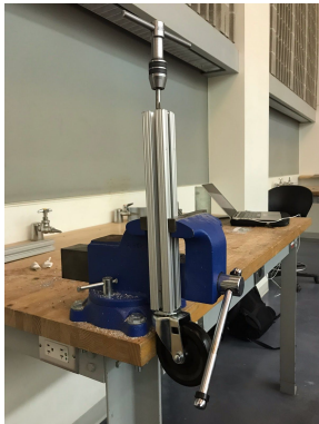
Figure 8: Tapping of the upper portion of the legs to allow for the attachment of the hinge. Hole for wheel has already been expanded and tapped, with wheel attached in image.
