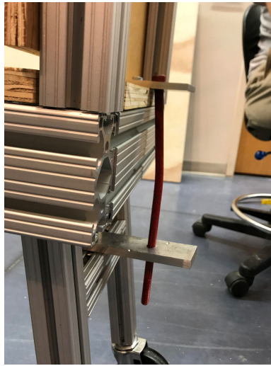
Figure 17 (left): The results of our initial test of the locking mechanism. The bolt shows significant bend and led to a redesign of the bolt.
