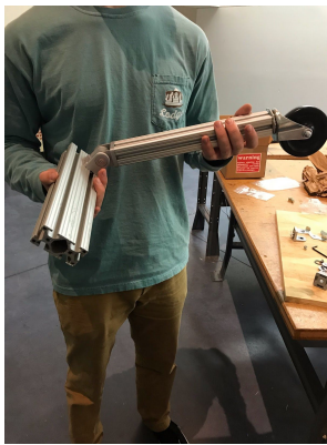
Figure 9: One of the rear legs attached to the back portion of the chair frame.
