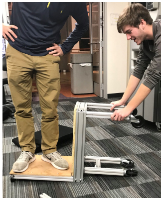
Figure 16: Impulse loading test using weight of team member
