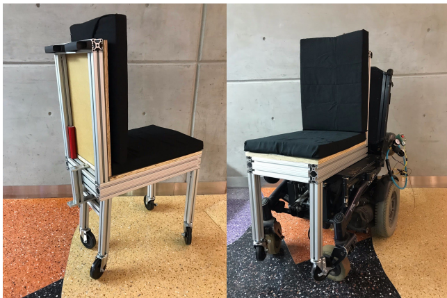
Figure 13 (left): Final design with rear wheels folded down
