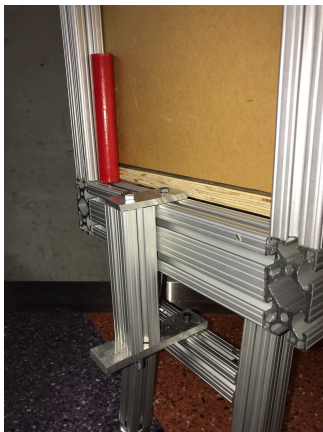
Figure 12: Completed final locking mechanism with attached holder in place.
