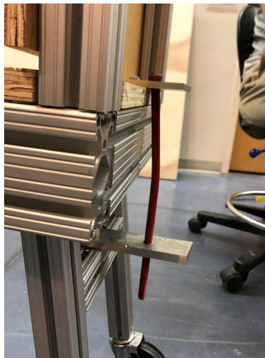
Figure 19 (left): The results of our initial test of the locking mechanism. The bolt shows significant bend and led to a redesign of the bolt.
