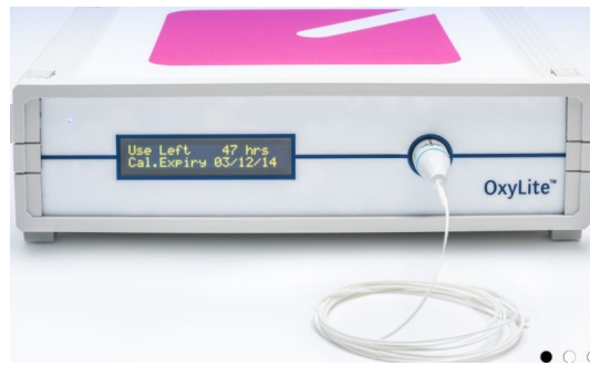
Figure 1: The OxyLite™ uses fiber optics in conjunction with a platinum-based fluorophore to obtain dissolved oxygen measurements in vivo .
