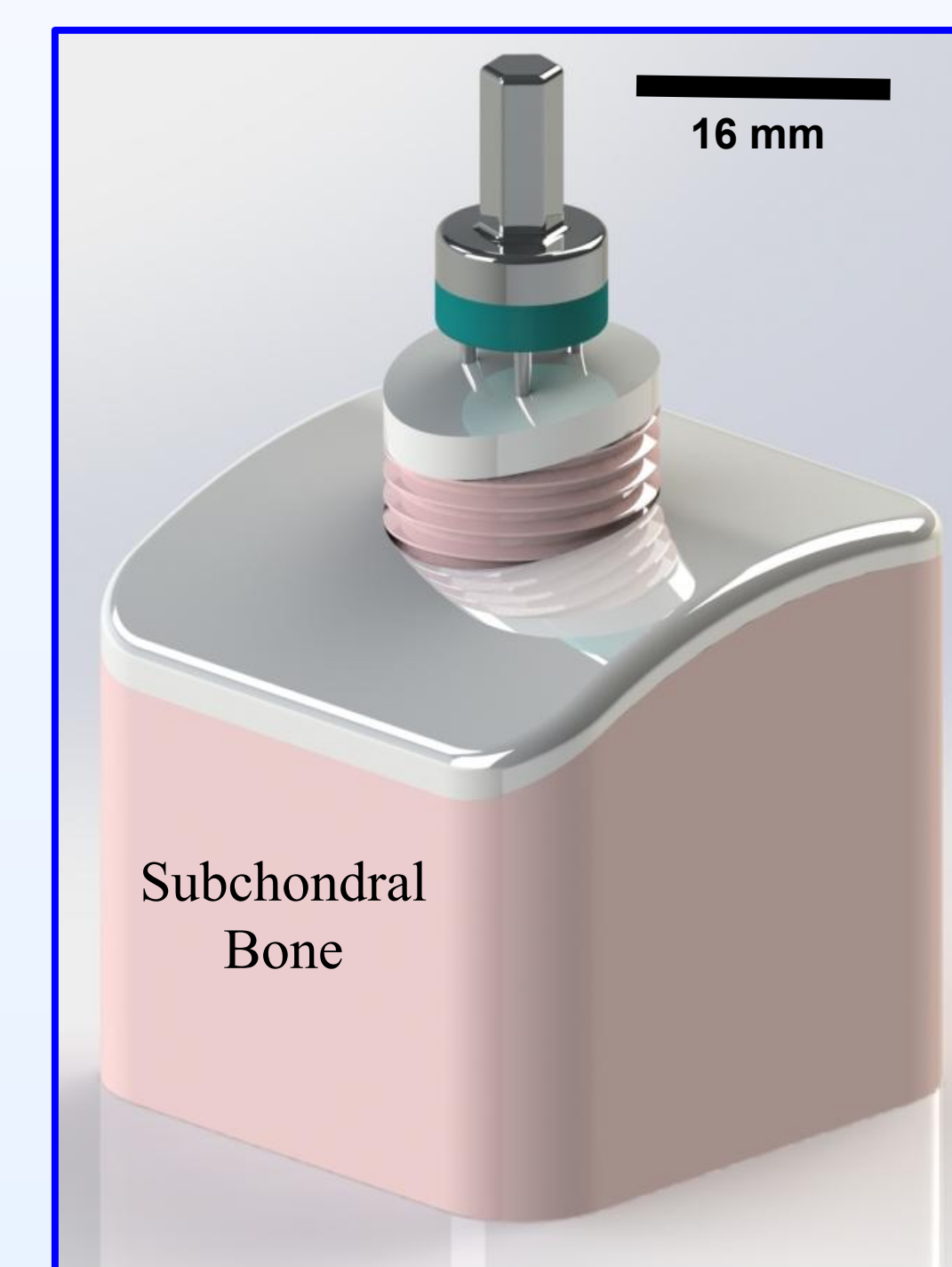
Figure 3: Solidworks rendering of graft screwdriver used to insert the allograft into the recipient site of the patient.
