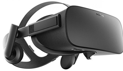
Figure 3: An Oculus Rift headset. Dimensions: 184 x 114 x 89 mm [30]
