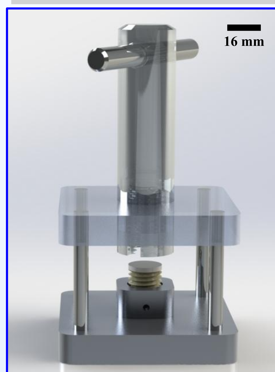
Figure 2: Graft threading fixture. The graft is fixed in supporting cup. The guiding platform ensures axial alignment between the graft and die to cut accurate threads.
