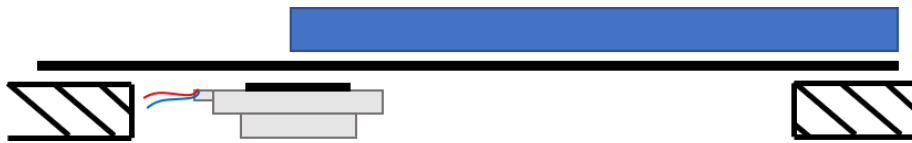
Figure 4. Testing setup of load cell test. The load cell (blue) is placed on either the vibrating pedal or the non-vibrating pedal. The force generated by the transducer is collected and analyzed.
