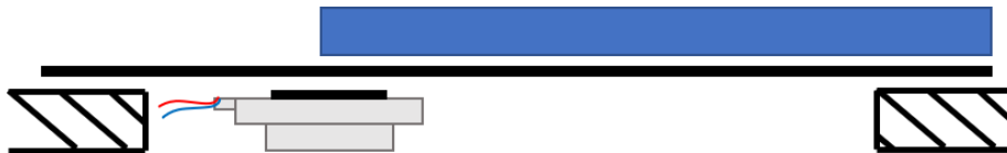
Figure 4. Testing setup of load cell test. The load cell (blue) is placed on either the vibrating pedal or the non-vibrating pedal. The force generated by the transducer is collected and analyzed.
