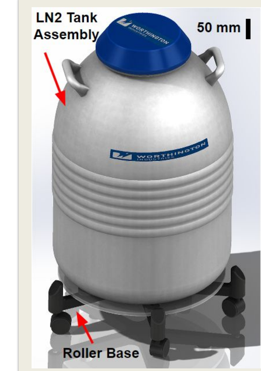
Figure 4: SolidWorks rendering of the fully assembled roller base and integrated scale with the LN 2 tank placed directly on the assembly
