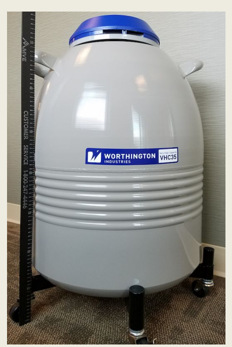
Figure 1: Worthington VHC35 LN 2 Storage Tank With Roller Base
