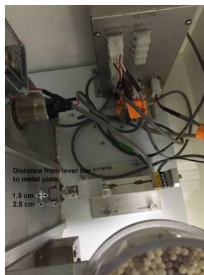
Figure 1: Picture of current system, handlebar will be 2.5 cm from the slot in the cage wall
