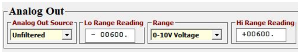
Image 27: The SST software settings that are required for accurately measuring force, when using the analog output.
