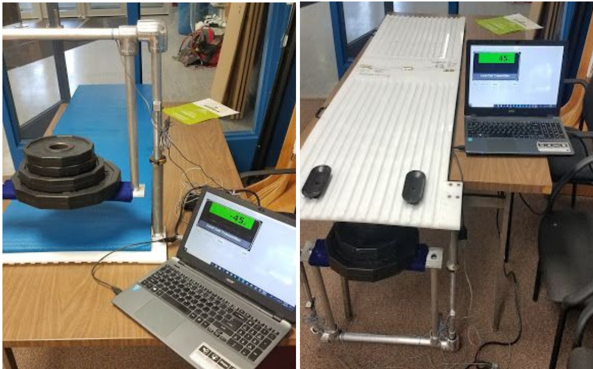
Image 28: Testing being performed in the Shell for both compression (right) and tension (left) values, with a weight of 45 pounds being applied in both instances.
