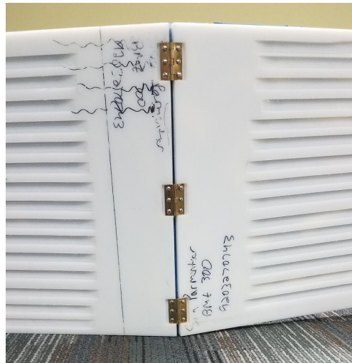
Image 9: A bottom view of the completed prototype, featuring the base plates and the dado cuts that were made into them to reduce their overall weight. Also shown are the affixed hinges and the milled pockets.
