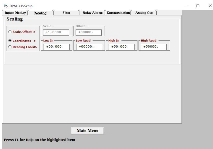
Image 22: Scaling screen, within which the input and output readings of the SST Transmitter could be adjusted [16].
