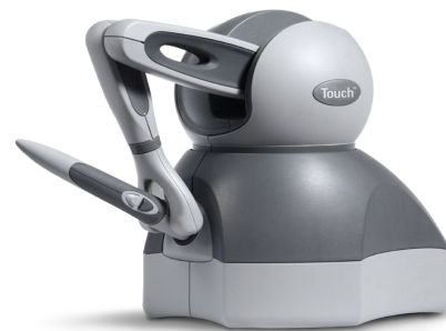
Fig.2 The image depicts a PHANToM Touch (3D Systems), comprised of a handheld stylus attached to a motor arm. The device interacts with an independent computer running Geomagic software via USB 28 .
