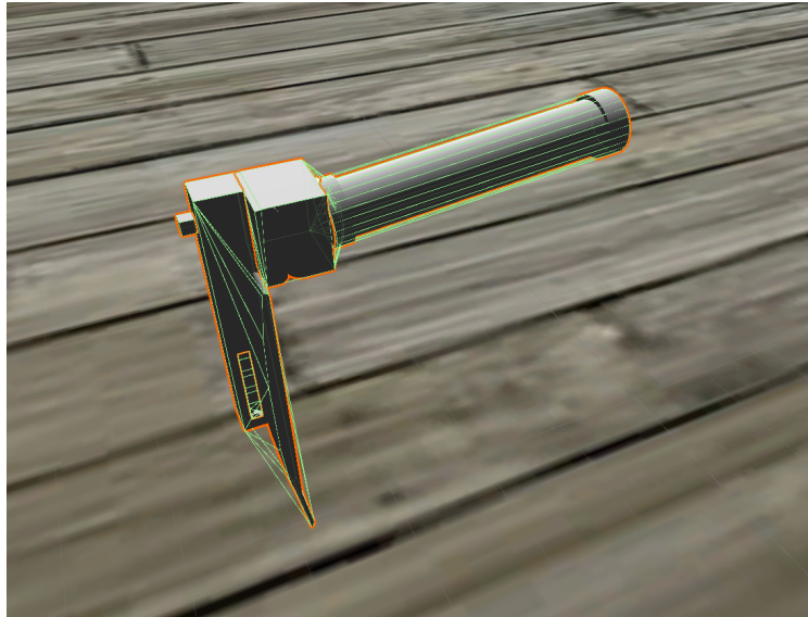
Figure 31: Unity uses a system of meshes to calculate collision physics, parsing the object into triangles, as pictured above. The described haptic software will calculate collisions based on evenly distributed points along the surface of the tool.
