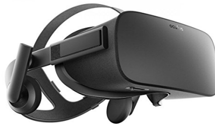
Figure 2: An Oculus Rift headset. Dimensions: 184 x 114 x 89 mm 38)
