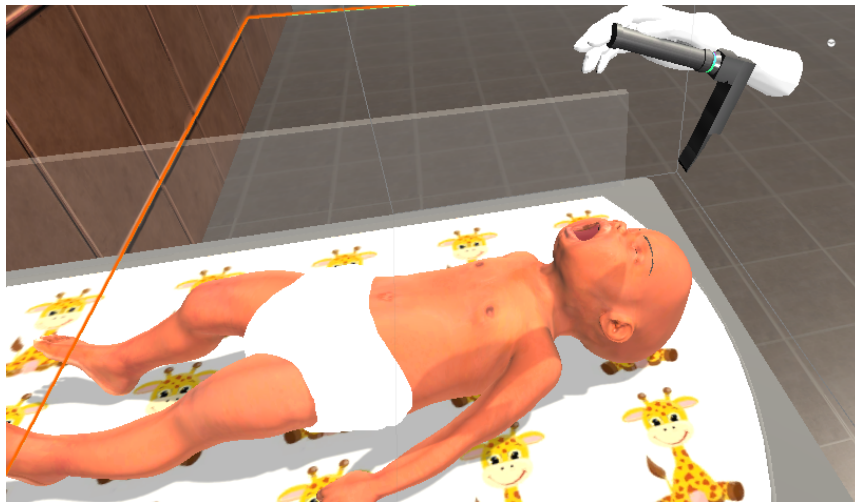
Figure 38: All of the previously described 3D models were incorporated into the Unity scene for the first time. The neonate rests upon the GE Giraffe model, as it would in a real procedure. Further, the haptic device controls a hand that can grab the laryngoscope blade, which can then interact with the neonate.
