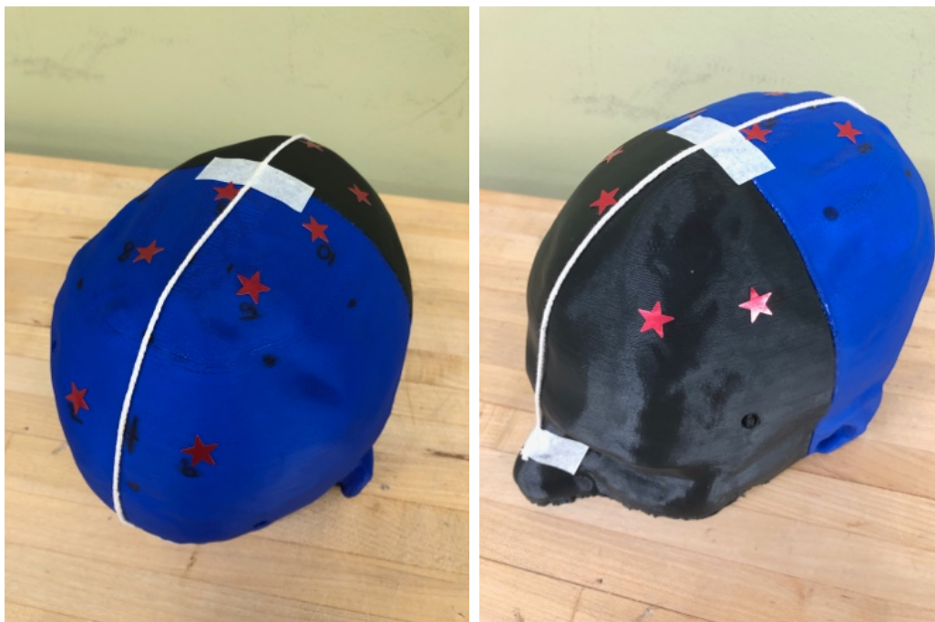
FIGURE IV and V. Pictured above is the head finalized and glued together. Stars represent the holes used for testing the accuracy of gyration later.
