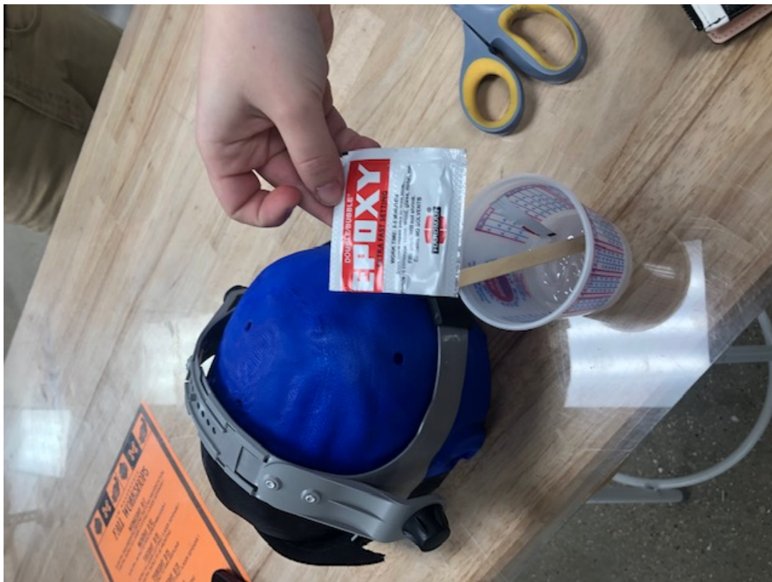
FIGURE III. Epoxy glue was utilized in order to fasten the two halves of the print. Gyration was placed on the model after Epoxy application to ensure that the halves stuck together.
