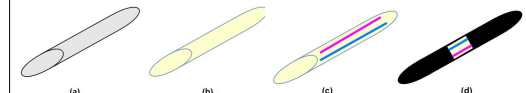
Figure 9: Four step process for electrode delivery (a) typical catheter (b) Adhesive coating (c) Electrodes adhered to catheter (d) Insulating layer
