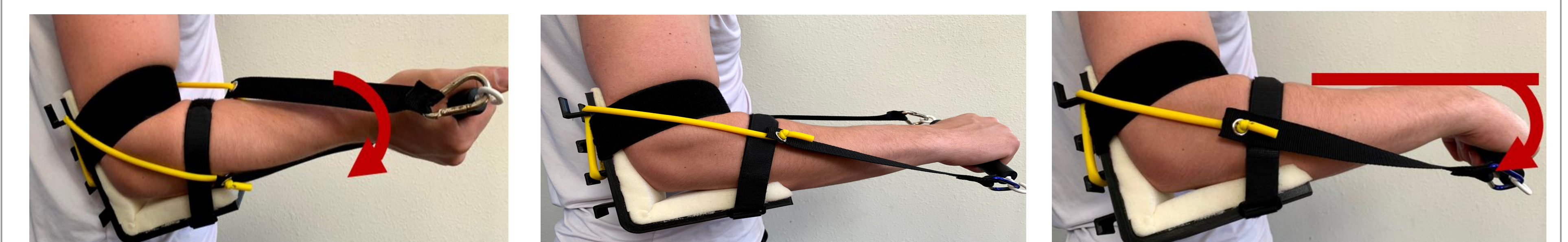
Figure 12: Forearm motions used with the device. Shown is the original design with updated resistance bands.
