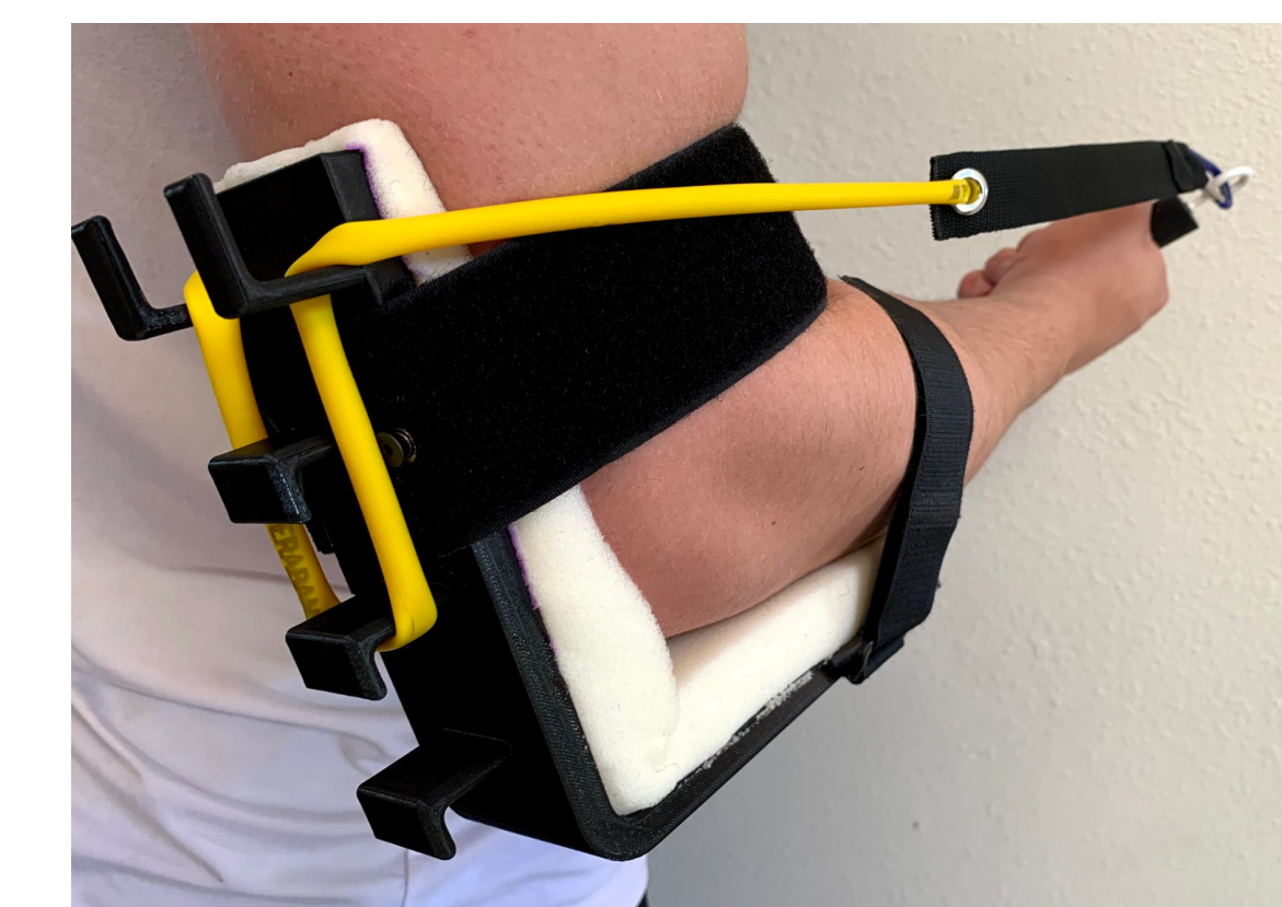
Figure 7: Original design with updated resistance bands
