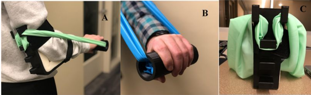
Figure 7: Pictures of three different angles of the original design. Image A is an isometric view of the design. Image B shows the handle. Image C depicts the back of the design, showing the adjustable resistance hooks.
