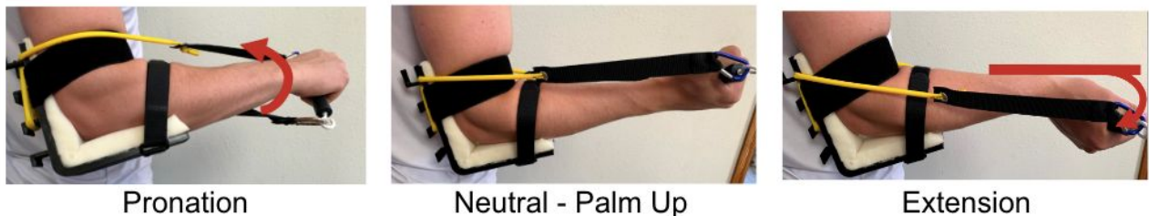
Figure 22: Forearm motions for extension and pronation that can be performed with the device.
