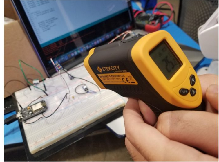
Fig. 11: A-B , The temperature at the bottom of the breakout board was measured using an infrared laser heat gun.
