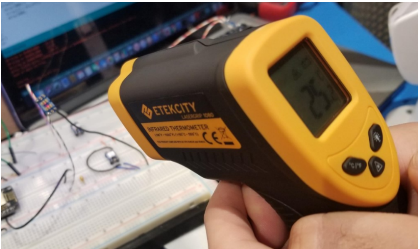
Figure 1: Image of the testing procedure. The LED was connected to a breadboard and suspended with the breakout board facing us. An infrared laser heat gun was used to measure the temperature.
