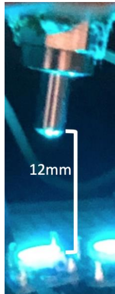
Figure 8: The testing schema of light intensity using the Ocean Optics Spectrophotometer USB2000+.
