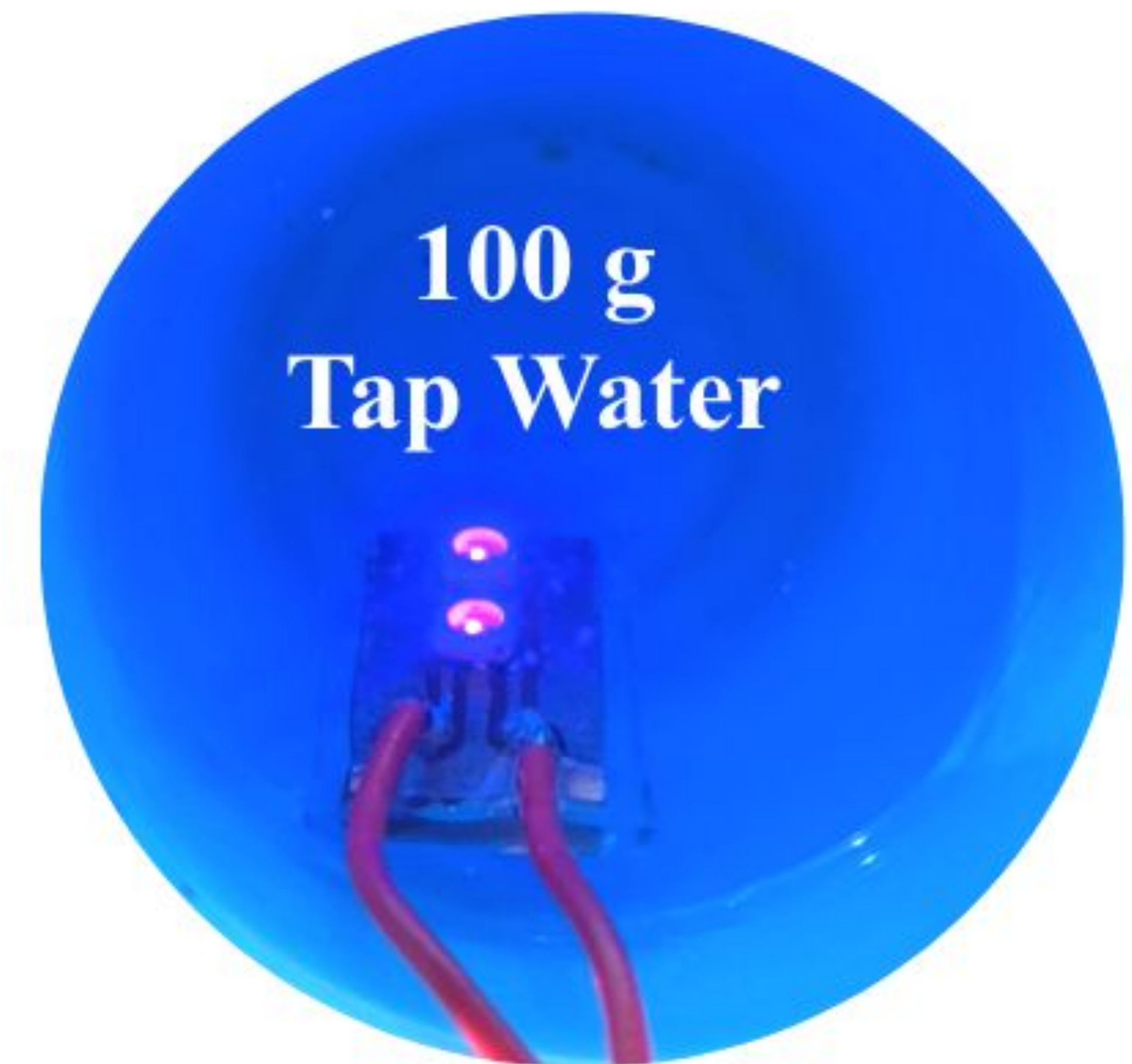
Figure 4. LED Temperature Testing. Change in temperature of the water containing the coated 465 nm LED was not statistically significant from the control ( p=0.086 ). Change in temperature of the water containing the coated 405 nm LED was statistically significant from the control ( p=0.049 ), however, LED is still within design specifications.
