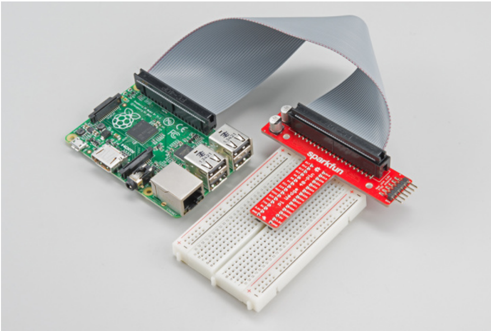
Figure 2: Raspberry Pi connected with I 2 C
