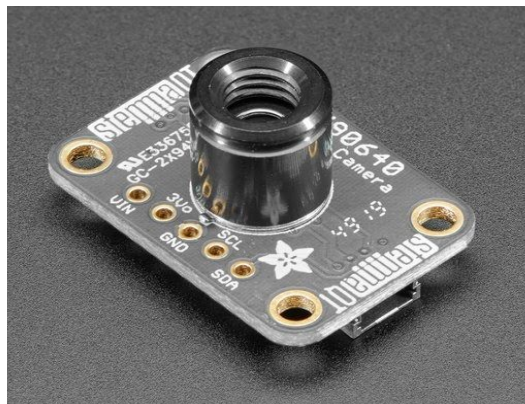
Figure 8. Image of the MLX90640 thermal camera. This camera provided the best imaging quality for a price that fell within our Budget.
