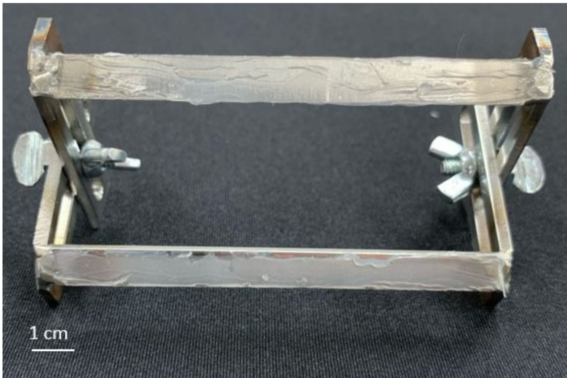
Figure 4, Initial Design. Bottom view of prototype displaying the thin silicone adhesive layer.
