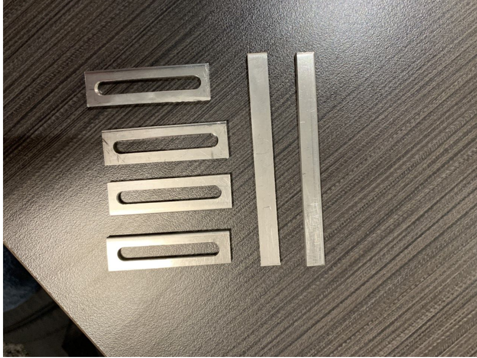
Figure 13, Material Components. Separated stainless steel pieces after waterjet cutting which will form the final design.
