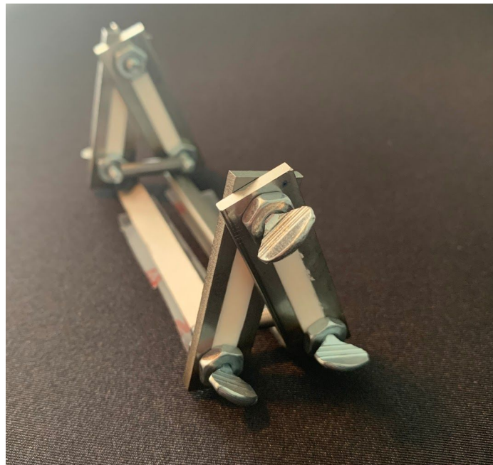
Figure 5, Improved Final Design. Image portraying the final design improvement including the tension springs and the 3D printed slot fillers.
