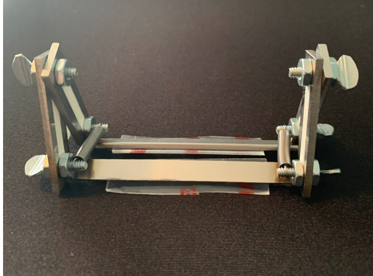
Figure 6, Improved Final Design. Image portraying the final design improvement including the tension springs and the 3D printed slot fillers.
