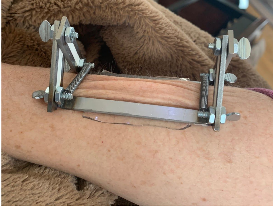
Figure 6, Device in Service. Final design in service on human skin. The skin was pinched until raised to simulate approximation of wound edges.
