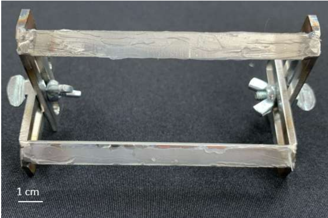
Figure 15, Final Design. Bottom view of prototype displaying the thin silicone adhesive layer.
