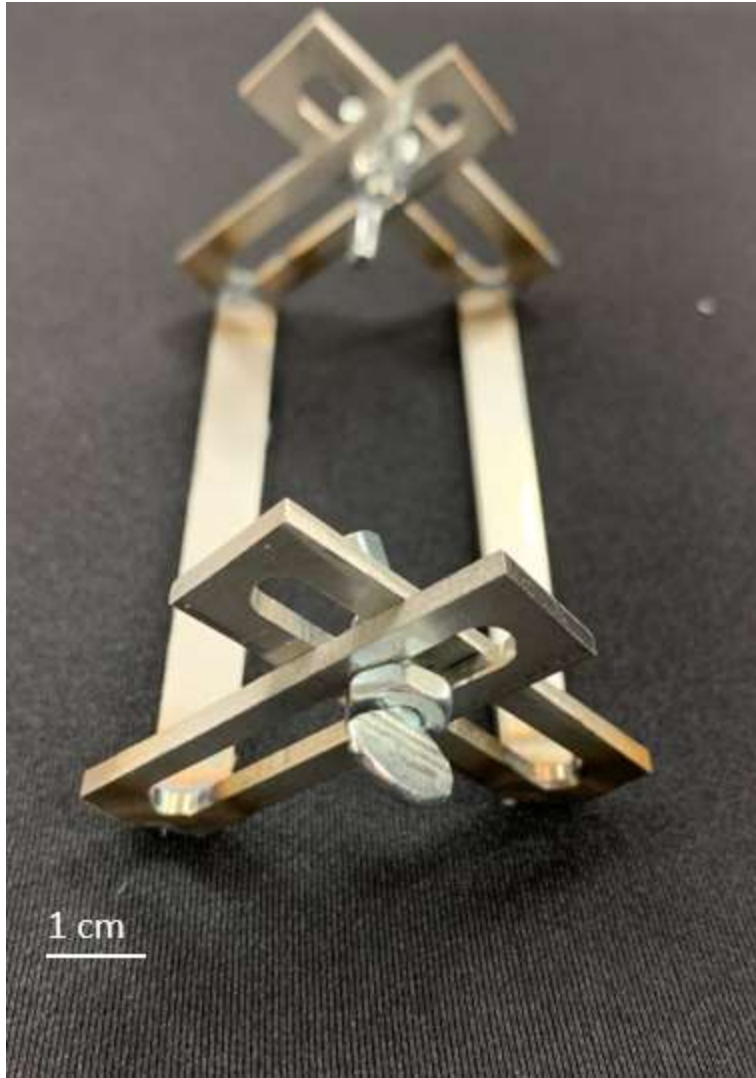
Figure 14, Final Design. Side view of assembled prototype including the fastening mechanism, thumb screws.
