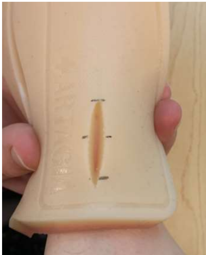
Figure 19, Silicone Laceration. The laceration made on the silicone skin for testing. The skin was then draped over a forearm to cause the wound edges to splay.
