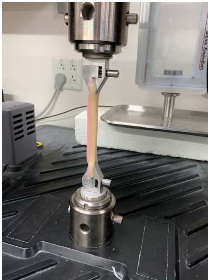
Figure 18, MTS Testing. Image of the silicone skin strips in the MTS grips during tensile testing. The specimen was exposed to axial tension until the silicone began to slip from the grips.
