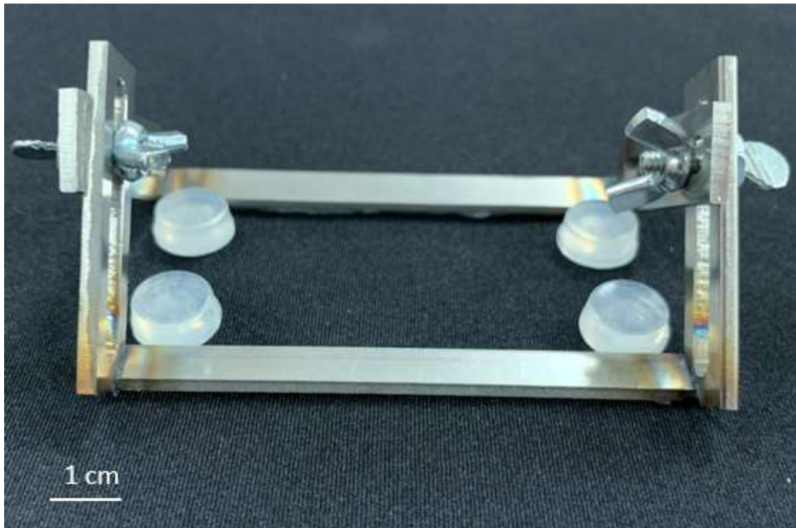
Figure 3, Final Design. Front view of prototype with four silicone bumpers used during wound edge approximation.
