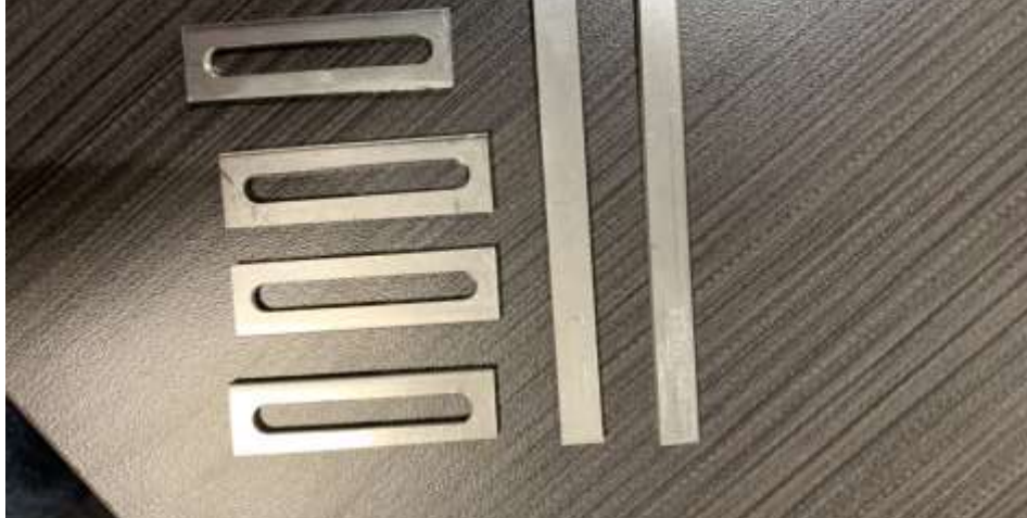
Figure 13, Material Components. Separated stainless steel pieces after waterjet cutting which will form the final design.
