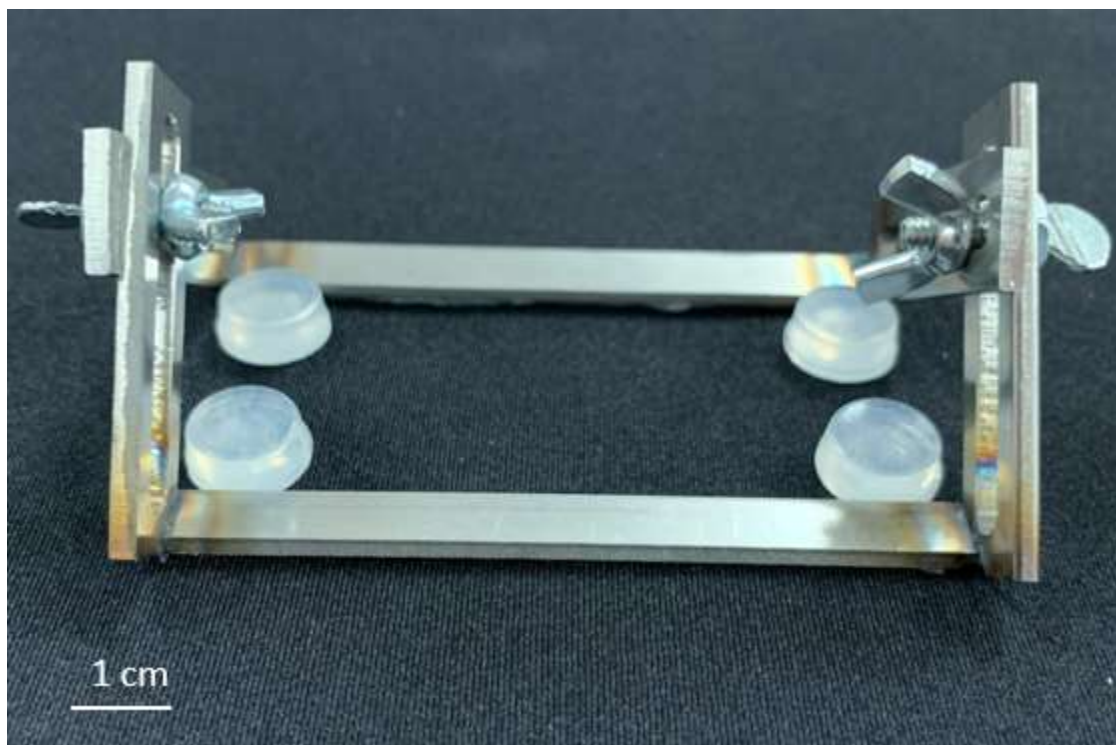
Figure 16, Final Design. Front view of prototype with four silicone bumpers used during wound edge approximation.
