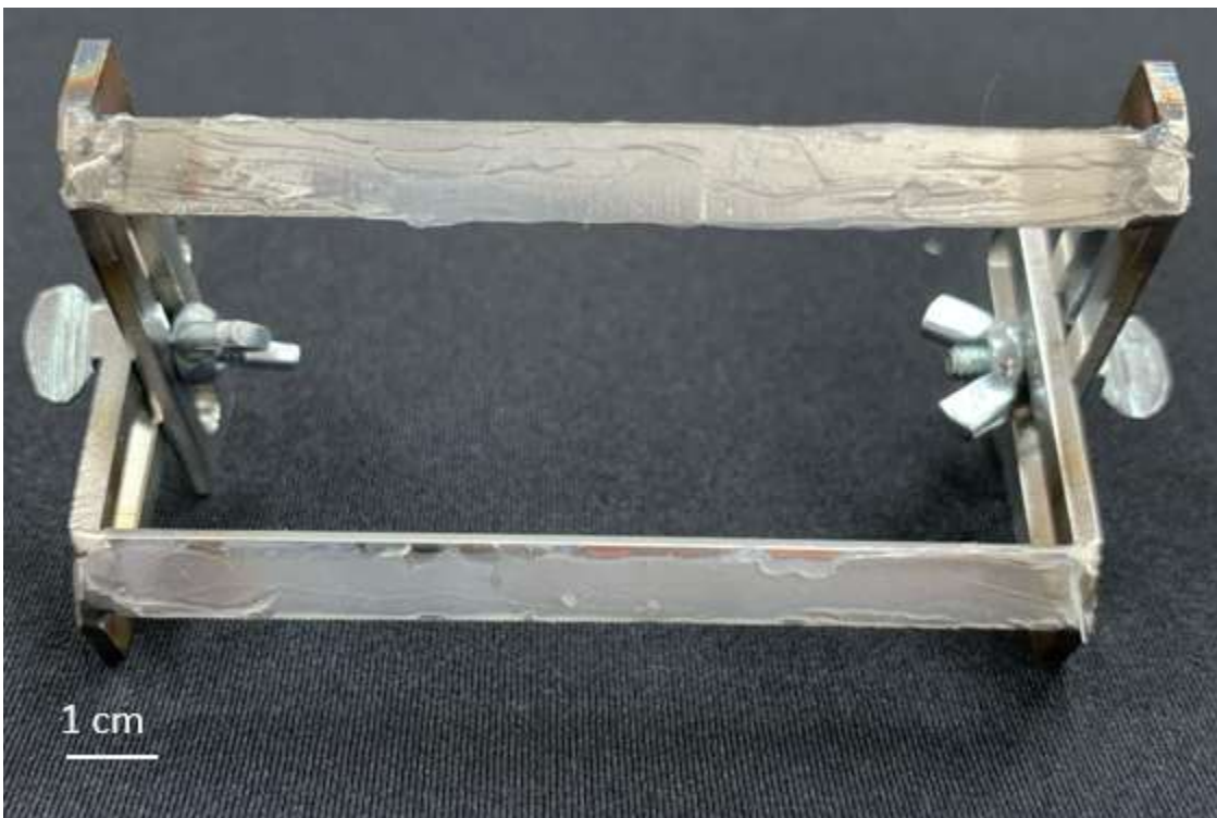
Figure 4, Final Design. Bottom view of prototype displaying the thin silicone adhesive layer.
