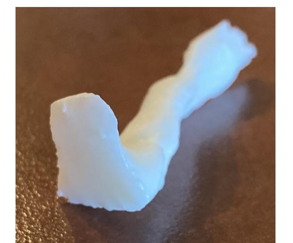
Figure 6.2 3D printed result of ear canal. Printed with PLA.
