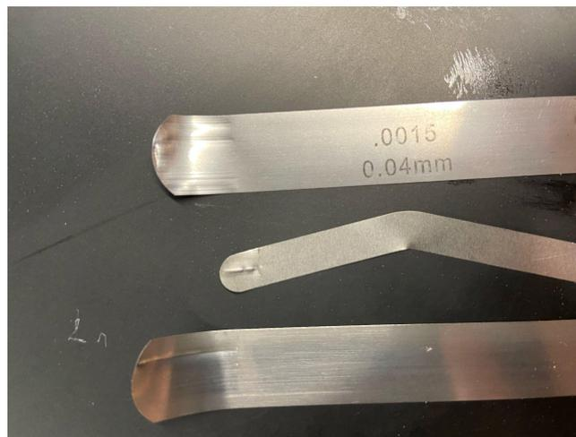
**Figure 5:** 0.0015 in feeler gauge, 0.0015in tofflemire bands, and 0.002 in feeler gauge (top to bottom) post testing in MTS machine.
