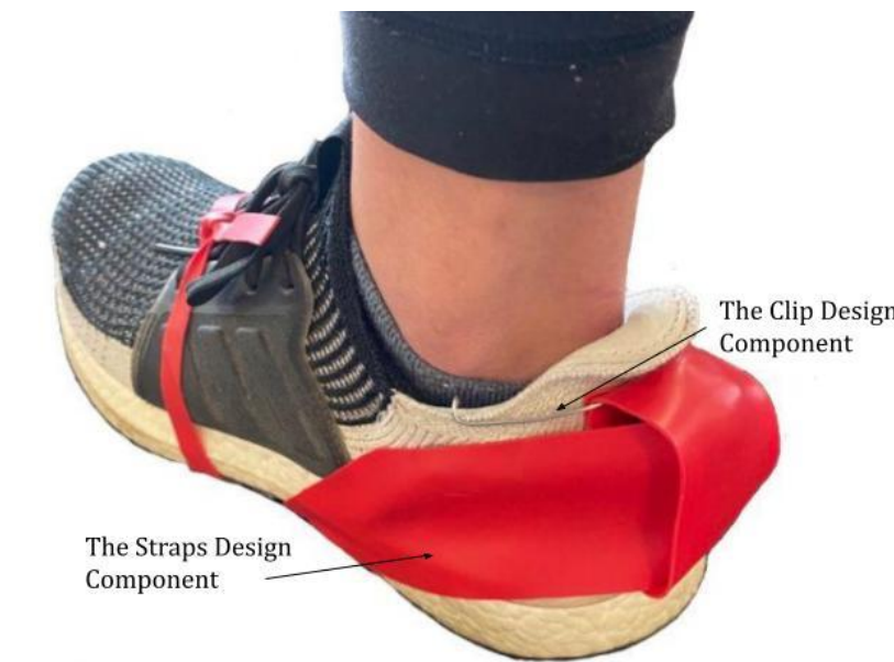
Figure 3: The complete shoe holder design with a latex strap and clip design to reduce movement in all directions.
