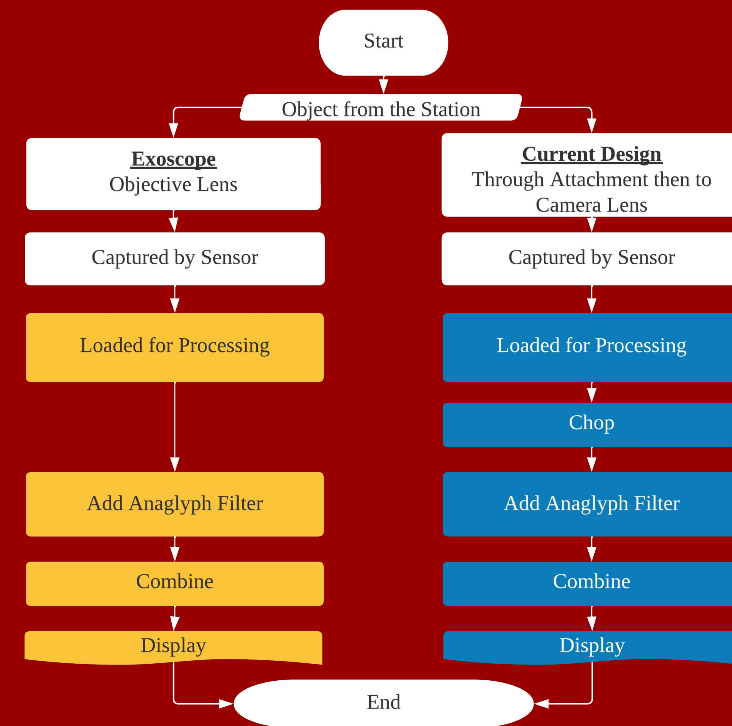
Figure 3: Workflow for exoscope (left) [3], and the mirror attachment design (right). Speculated processes highlighted in yellow; future work in blue.
