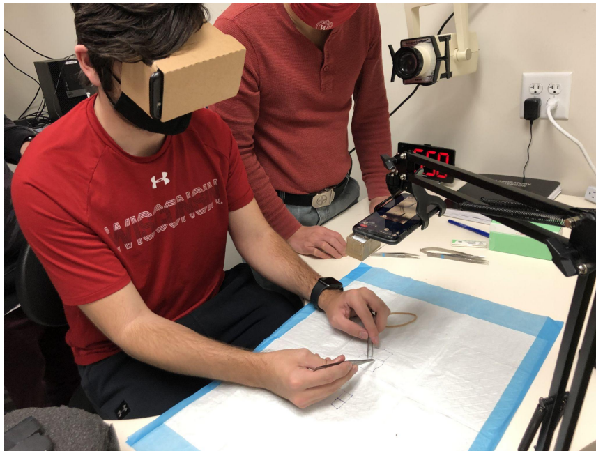
Figure 3: Testing the device using the Google Cardboard headset. The device can be seen attached to the smartphone that is mounted on the boom arm.
