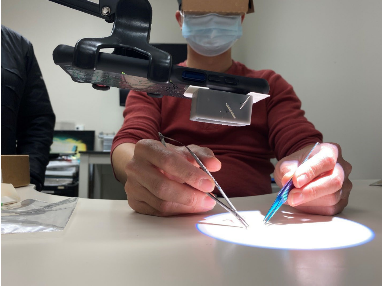
Figure 11: A client testing with the prototype. He tries to move two tweezers around to check out the depth perception. The client is wearing Google Cardboard, in which a smartphone displays the view recorded by the other smartphone that is above the station via Zoom. The second device is at 2x magnification, and the mirrors are fine-tuned to form clear image on the smartphone screen.
