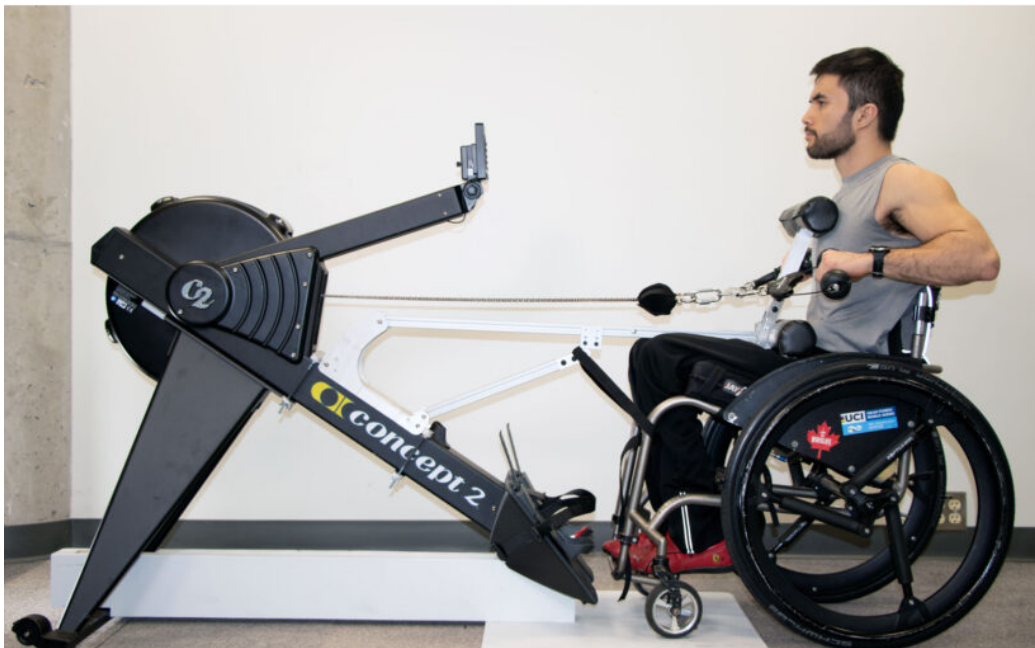
Figure 1. AROW adaptations to Concept 2. Adaptations for the Concept 2 include a support bar extending to the users chest and a rigid attachment to the frame of the rower [5].
