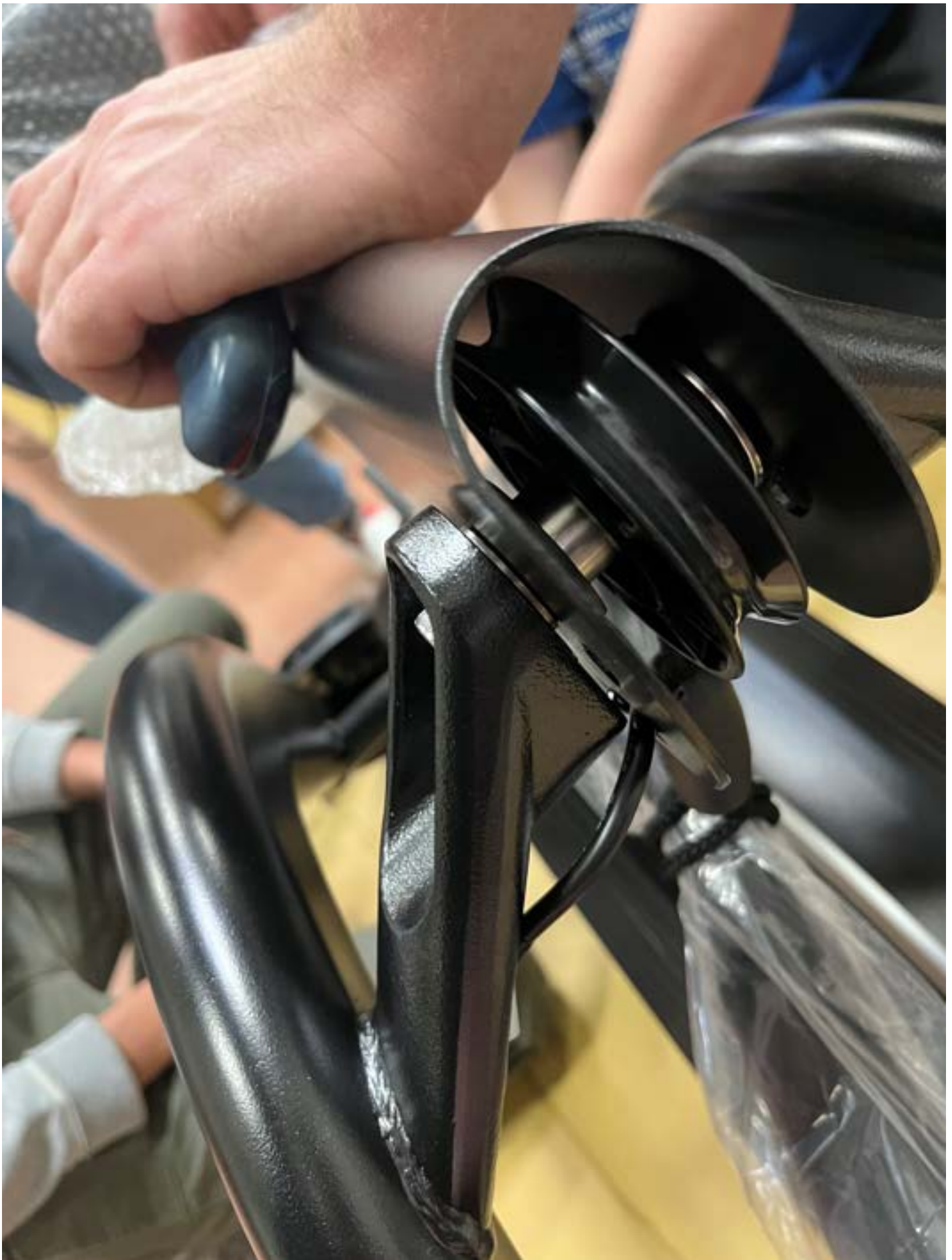
The above image shows the pulley that the rope wraps around in the support neck of the rower.
