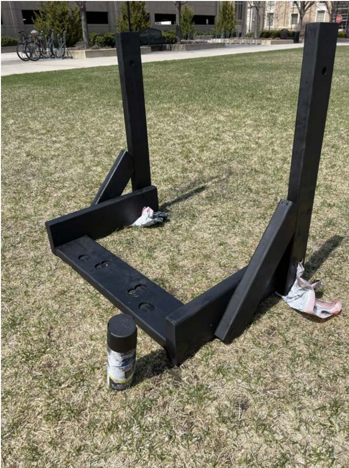
Figure 4: Second coat of spray paint
