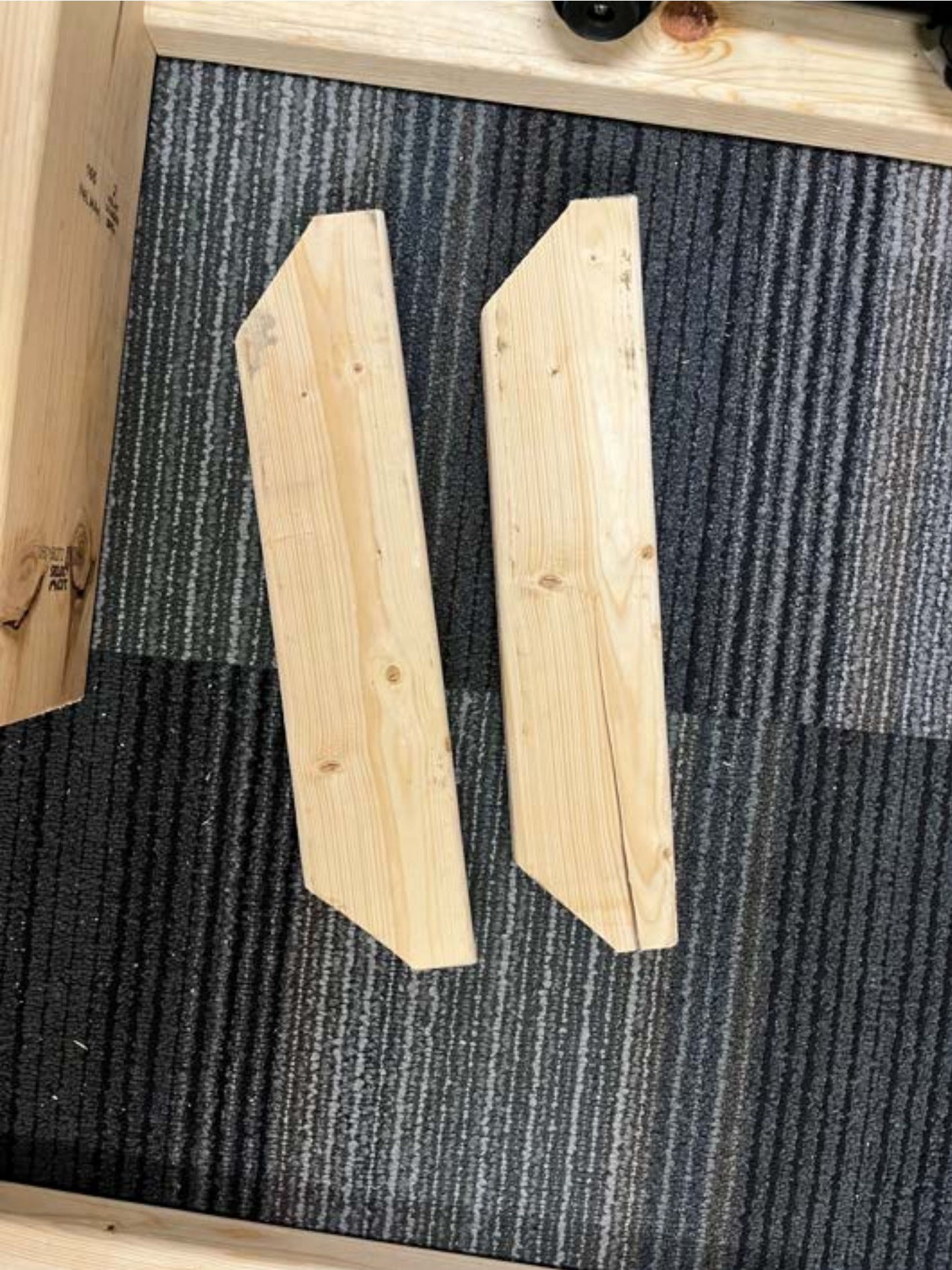
The above image shows the wood I cut. Ideally, the angled cut should have gone all the way to the corner.
