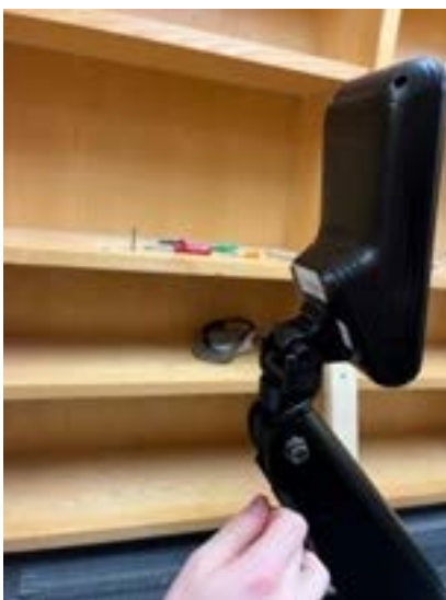
The above image is a back view of the swivel bracket with console attached.
