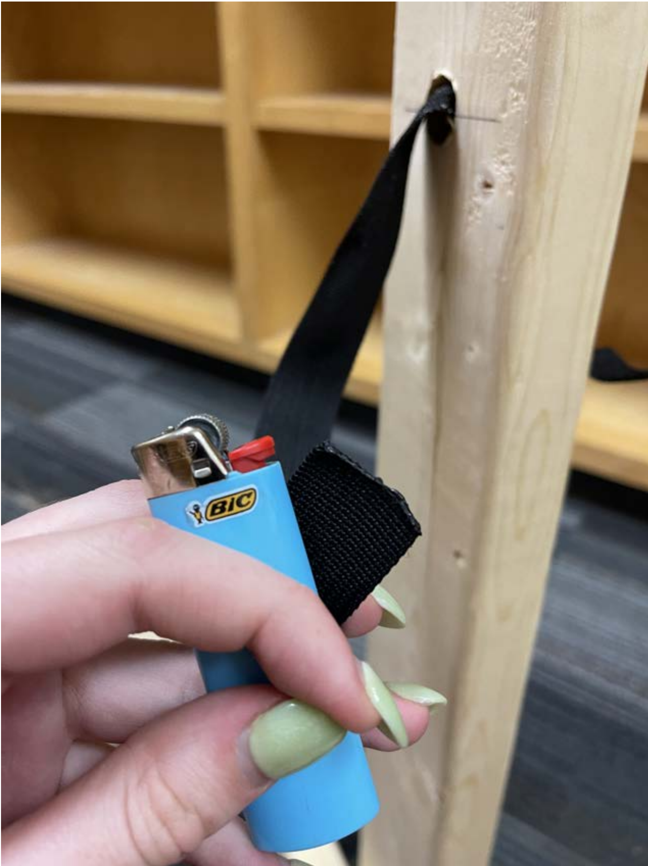
Figure 1: Strap end after exposed to lighter to prevent fraying
