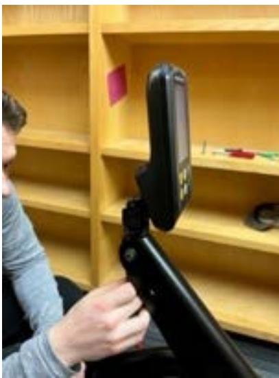
The above image is a side view of the swivel bracket with the display attached.
