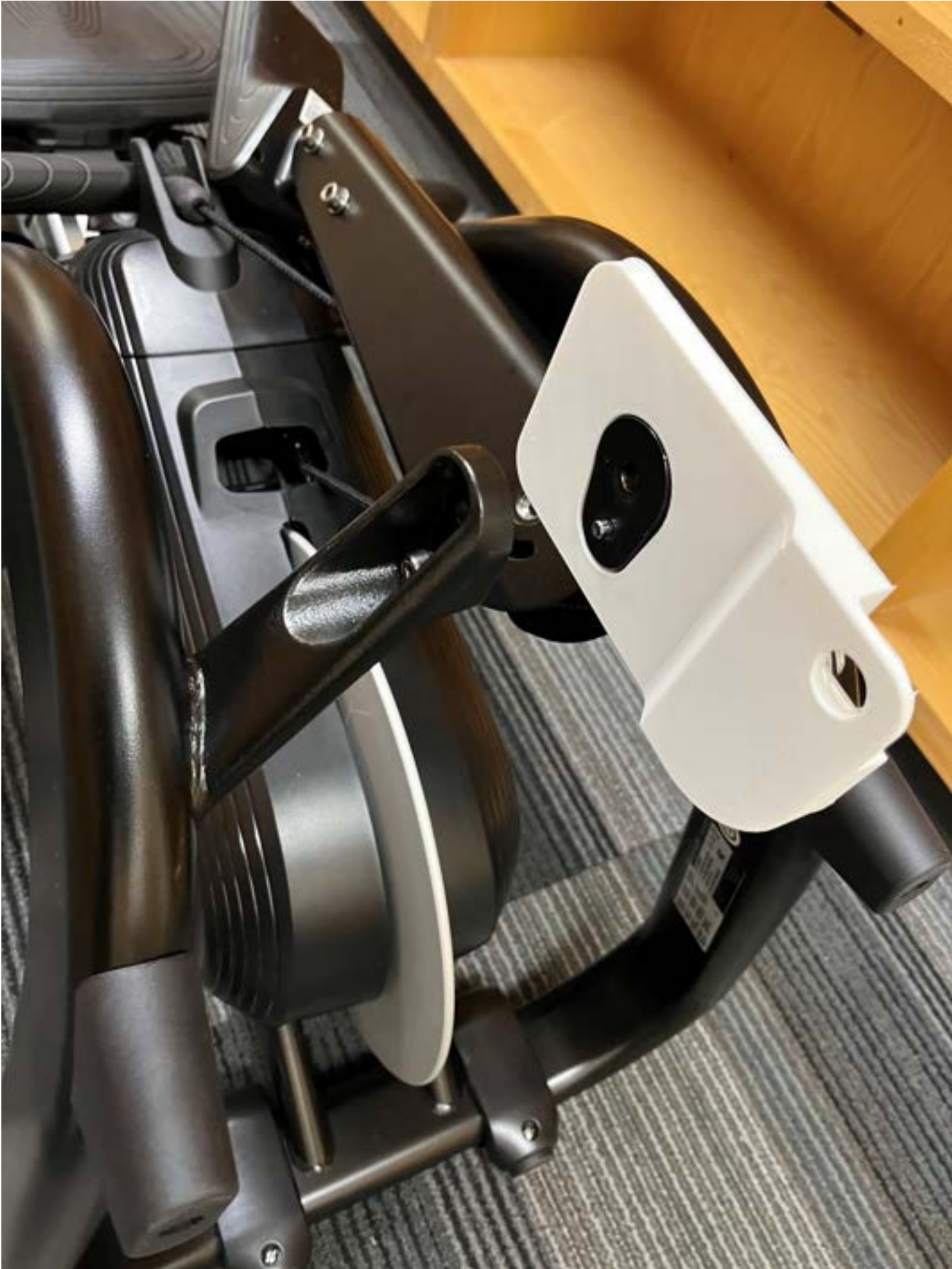
The above image shows the top view of the pulley plate on the rower.
