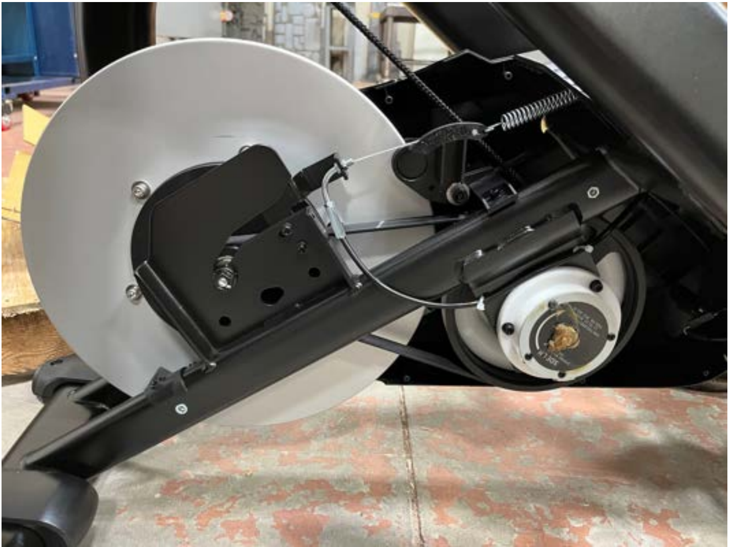
The above image shows the inner mechanism of the magnetic rower, including a flywheel, belt loop, and rope spool.
