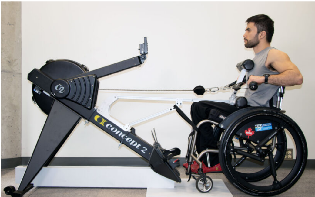
Figure 1. AROW adaptations to Concept 2. Adaptations for the Concept 2 include a support bar extending to the users chest and a rigid attachment to the frame of the rower.
