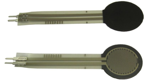
Figure 7: FSR 400 Force Sensing Resistor highlighting its two prong connectors that allow breadboard and circuit integration [Electronics, 2021].
