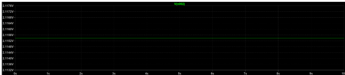
Figure 3: LTSpice simulation of the V_{out} from a voltage divider circuit containing a 3\text{ k}\Omega resistor for R_1 and a 2.2\text{ k}\Omega resistor for R_2 . The voltage output is about 2.115\text{ V} which can be estimated as 2.12\text{ V} .
