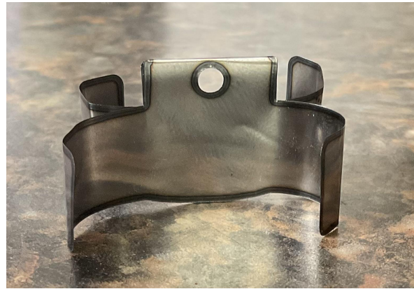
Figure 11: Laser Cut Prototype. High fidelity model produced by a laser cutter. Take note of the convex, rounded bottom edge, smooth corners, and smooth edges.
