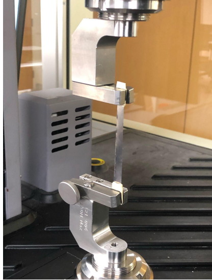
Sample being loaded into the MTS machine for tensile testing
