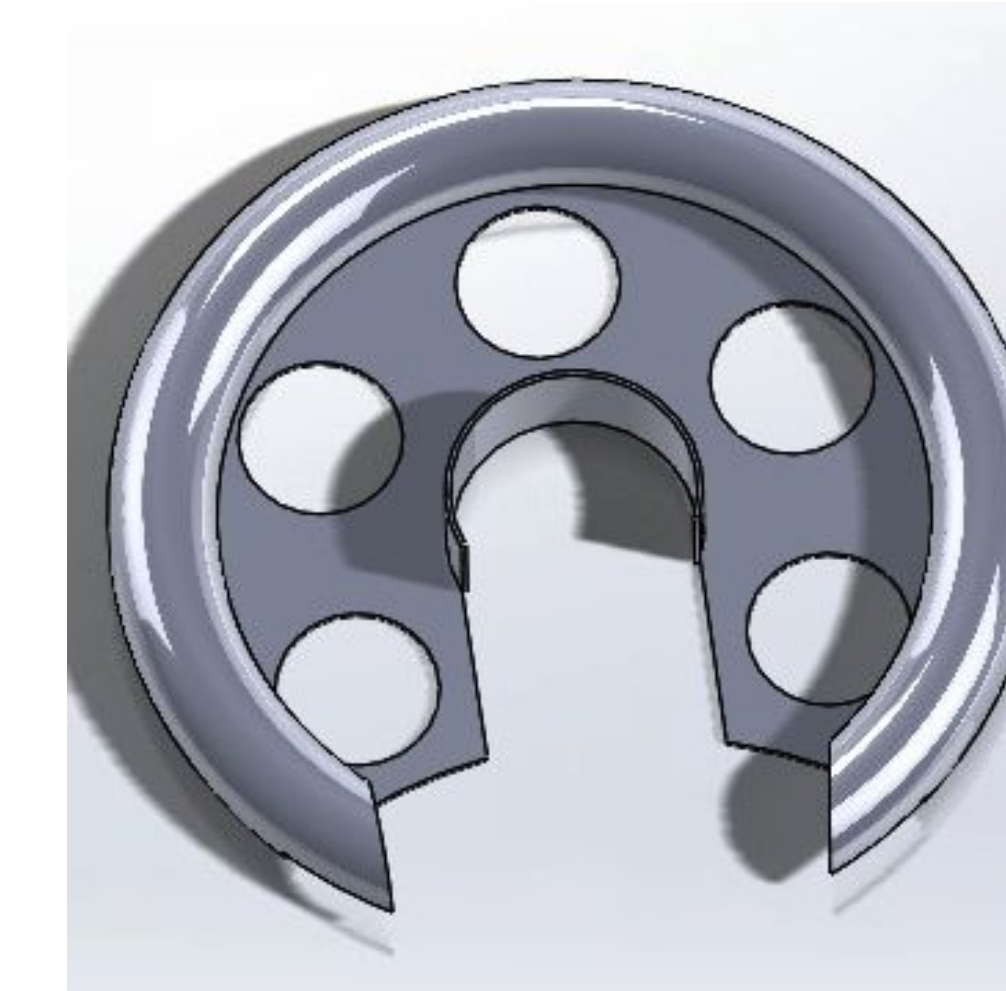
Figure 4. CutChimney Outer Diameter: 19cm, Chimney Diameter: 4.5cm
