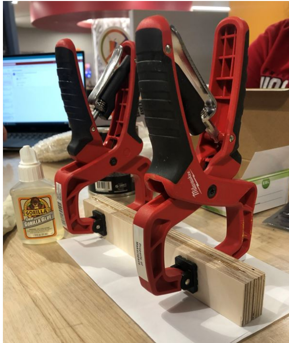
Figure 1: Two pieces of plywood being glued together to act as the core material for the model forearm. The strong core provided a backbone for the clay to be molded onto.
