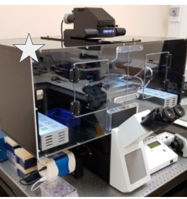
Figure 3: Elliot Scientific Stage-top incubator [3]
