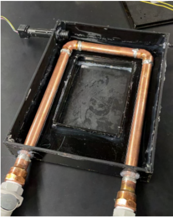
Figure 2: Photo of plumbing soldered copper tubing within the incubator box.
