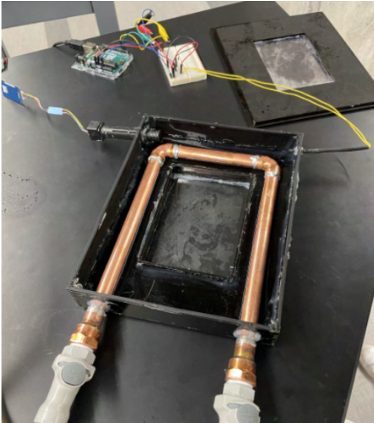
Figure 1: Final design fabrication with an open lid.
