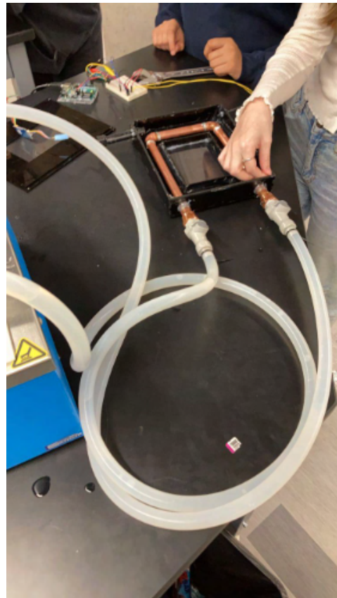
FIGURE 3: Leakage testing Setup
