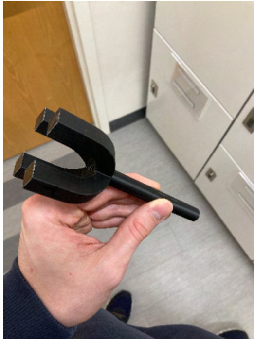
FIGURE 5: Final 3D Printed PLA Plastic Valve holder:
