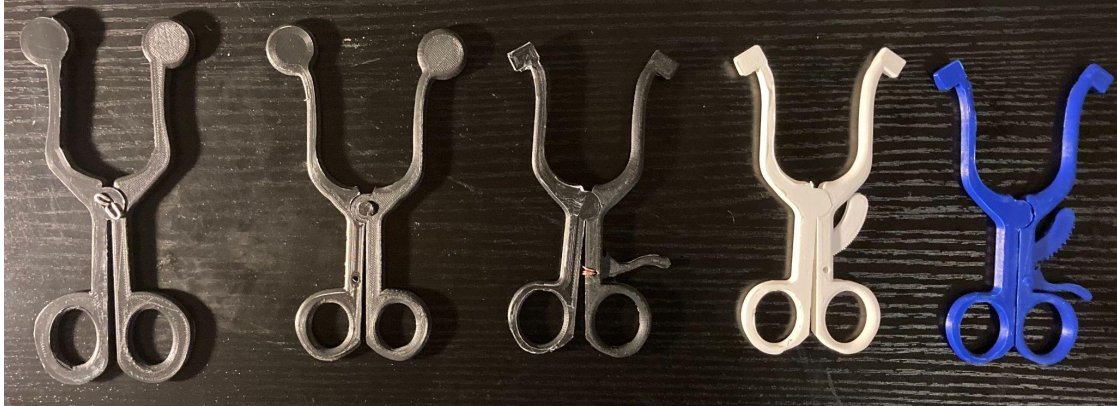
Figure 4: Five iterations of the device from the earliest (far left) to the most recent (far right).
